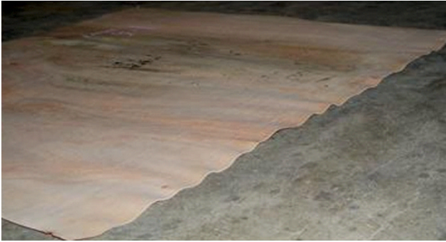
Figure 7. Frilling of veneer due to faster evaporation of moisture from the end grain of the veneer.
