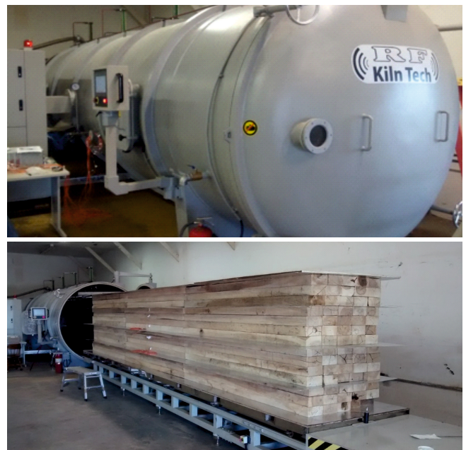
Figure 3. Commercial RF vacuum dryer at Silver Valley Custom Drying Upper Michigan USA
