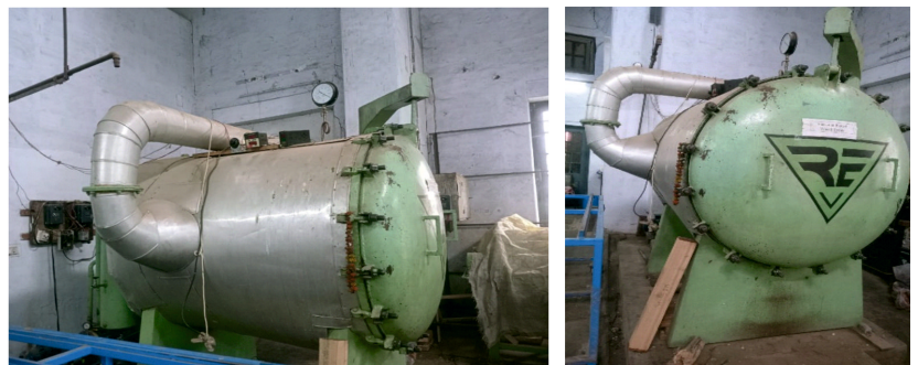
Figure 3 : Vacuum Dryer installed at wood Seasoning Discipline, Forest Products Division, FRI, Dehradun. (Vacuum Drying Technology patent by Dr. Nirmal Kumar Upreti, Wood Seasoning Discipline, Forest Products Division, Forest Research Institute, Dehradun. Patent Number: 349042)
