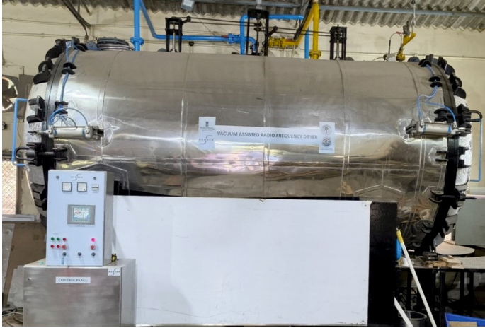
Figure 2. RFV dryer designed and fabricated by SAMEER, Mumbai
