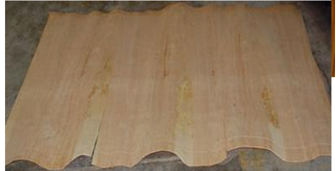
Figure 8. Buckling and splitting of veneers due to variation of initial moisture content across veneer surface
