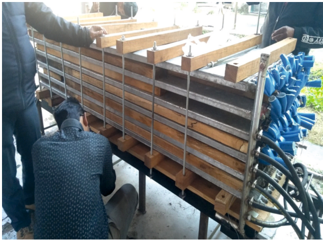
Figure 2: Stored heat is transferred to the platens through conduction
